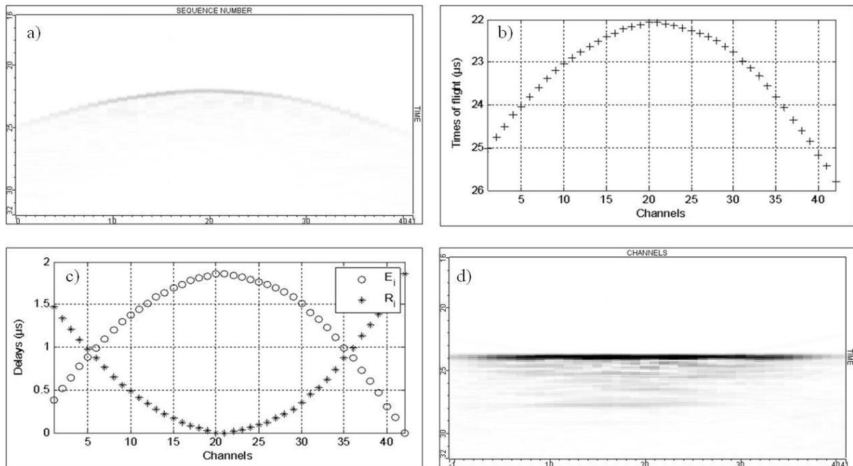
Figure 4: Adaptive process using an electronic scanning at emission: acquisition of the electronic B-scan (a); measurement of the specular times of flight (b); calculation of the emission and reception delay laws (c); transmission with all elements by applying these delay laws (d).
