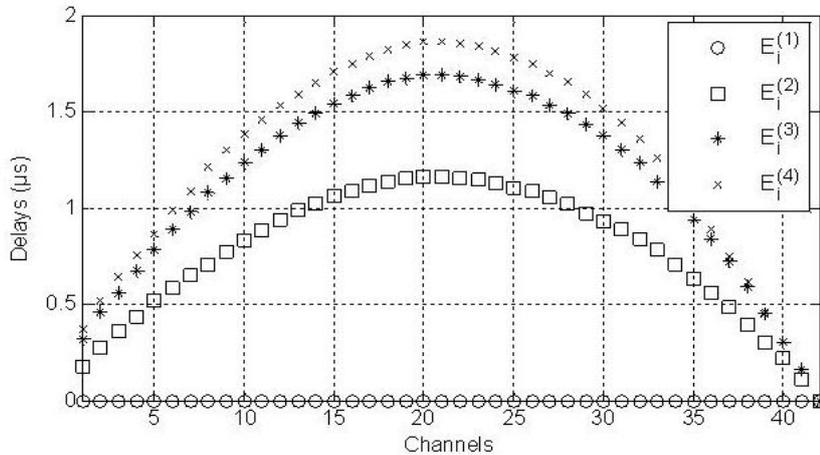
Figure 5: Successive emission delay laws applied in the iterative processing.
