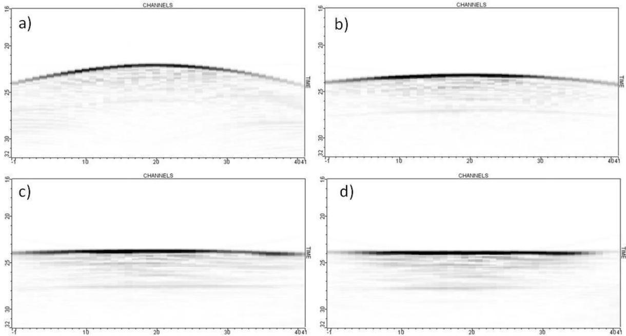
Figure 6: B-scans obtained for the successive shots of the iterative processing: first shot by applying  $E_i^{(1)}$  (a); second shot by applying  $E_i^{(2)}$  (b); third shot by applying  $E_i^{(3)}$  (c); fourth shot by applying  $E_i^{(4)}$  (d).
