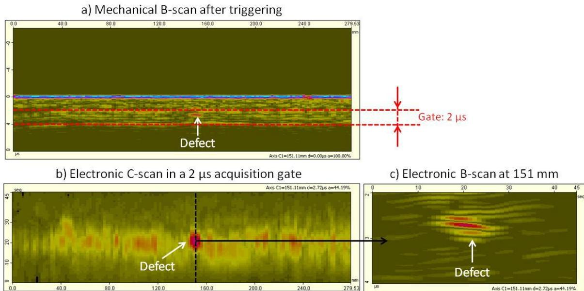
Figure 10: Mechanical B-scan after triggering for the 19<sup>th</sup> sequence (a); electronic C-scan with a 2 μs acquisition gate (b); electronic B-scan at the defect position (c).
