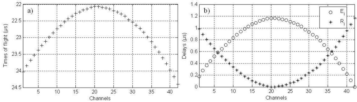
Figure 2: Times of flight measured from the front surface echo (a) and associated delay laws (b).
