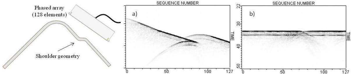
Figure 8: B-scans without processing (a) and by applying the SAUL algorithm with 3 shots (b).
