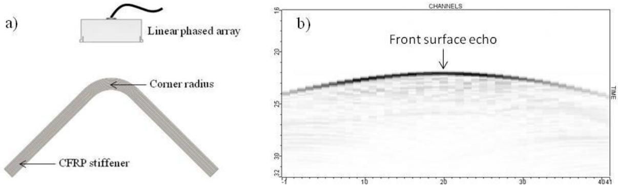
Figure 1: Experimental set-up (a) and typical B-scan obtained in paintbrush acquisition mode (b).
