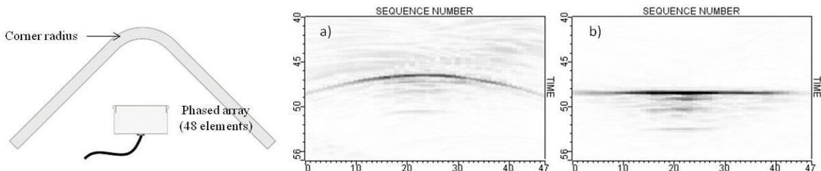
Figure 7: B-scans without processing (a) and by applying the SAUL algorithm with 5 shots (b).
