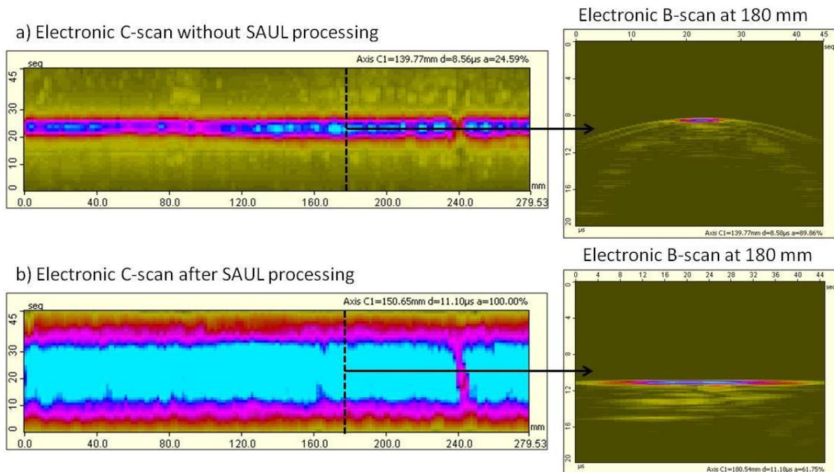
Figure 9: Electronic C-scans without processing (a) and by applying the SAUL function with 4 shots in each cycle of iterations (b).
